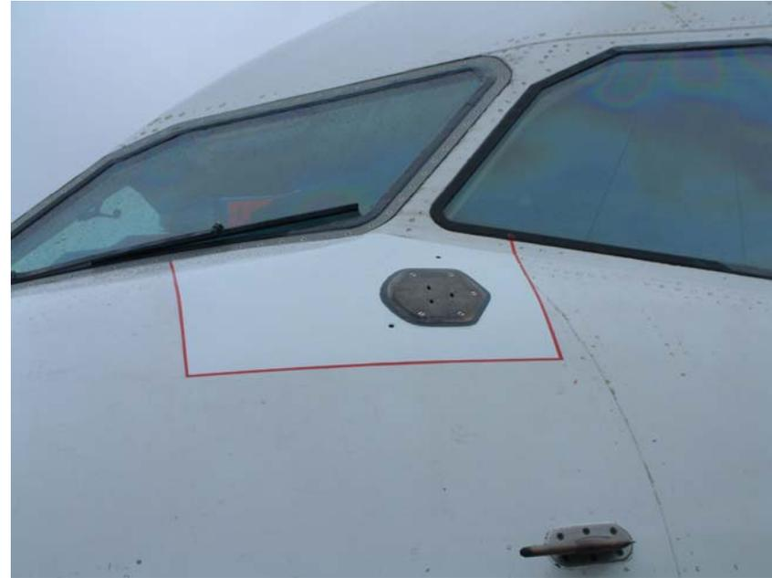
**within the marked area surrounding the left and right static plates as shown in the picture**
